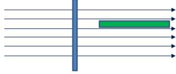
Least flux when plane of the surface is parallel to the field
