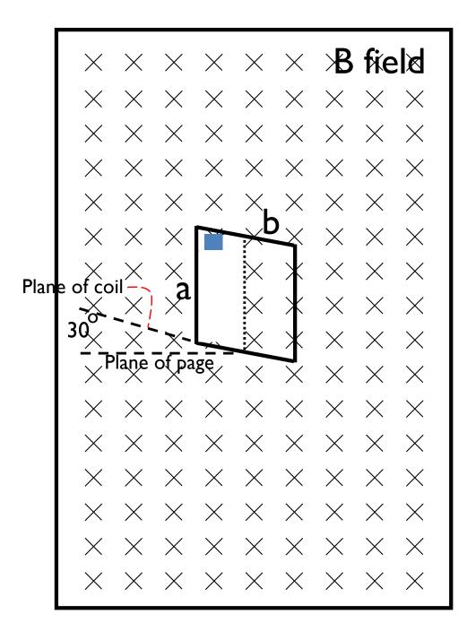
Same situation but with the coil rotated 30° into the page. What is the magnetic flux?
