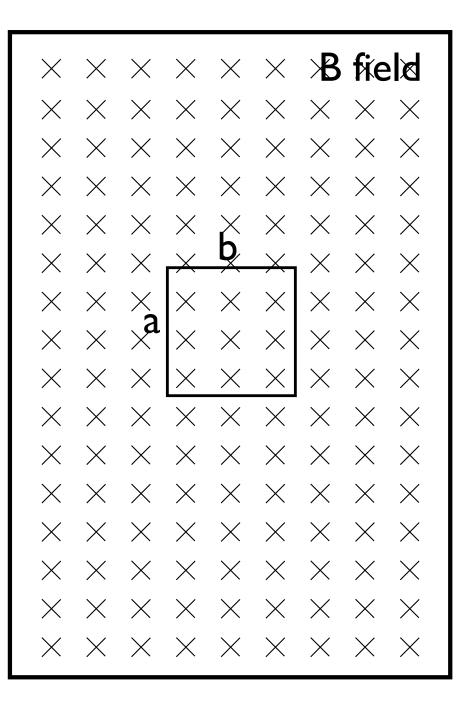
Assume you have a loop in the plane of the page that faces a magnetic field directed into the page. The dimensions of the loop are axb. Determine the magnetic flux through the coil.
